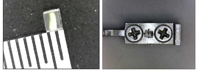
Fig. 6. (Left) Crystal target of ^{229}\text{Th}:\text{CaF}_2 . The size of the crystals is approximately 1 mm cubic. (Right) crystal holder. The crystal was attached to a target holder using a stainless steel fixing wire.
